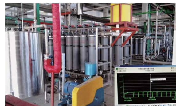
SMBR for alkali wastewater
