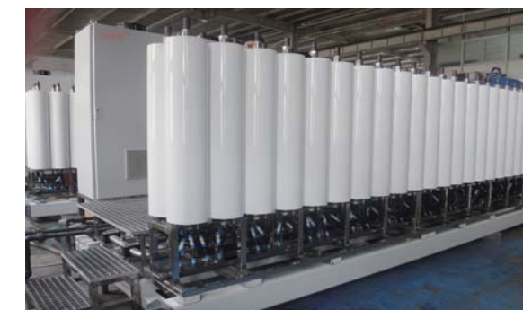
DTRO for leachate wastewater
